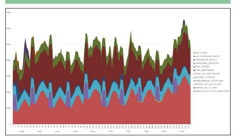
Figure 6. Total Hourly Gas Plant Curtailments by Type
