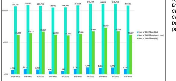
Figure 8. Total Daily Emissions from CEMS-tracked California Gas Plants During the Heatwave (8/31/22-9/9/22)<sup>27</sup>
