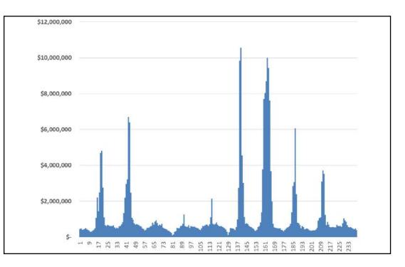
Figure 7. Estimated Hourly Value of Foregone Generation from Gas Outages and Derates. Value of lost gas generation totals \$283M
