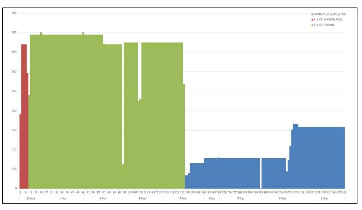
Figure 30. Total hourly curtailments by type for Ormond Beach Generating Station during the heatwave
