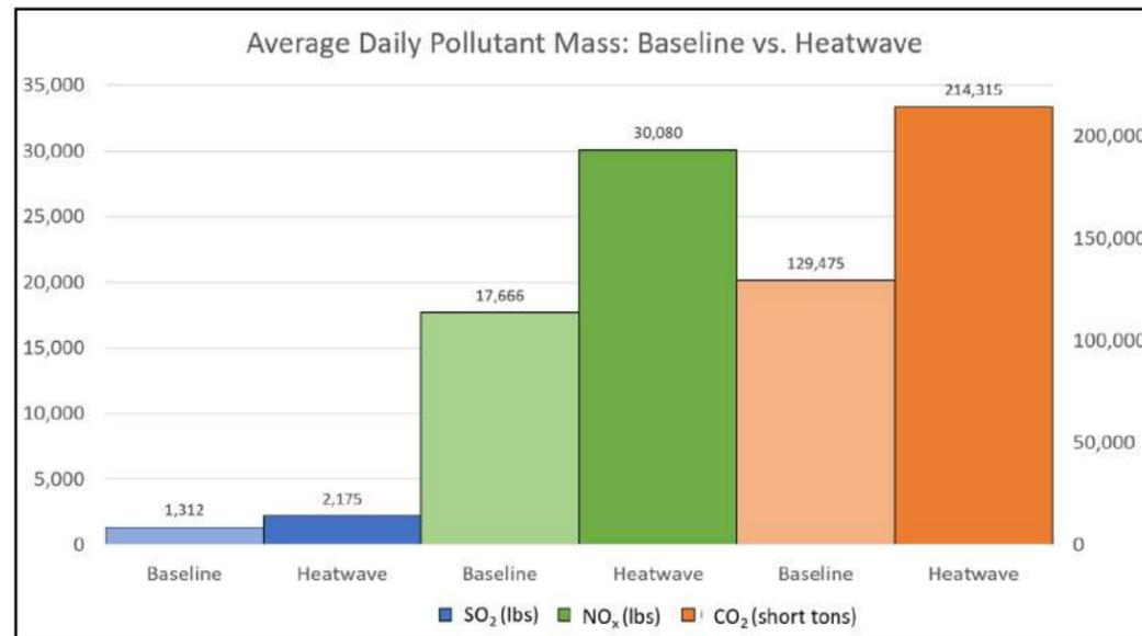
Figure 1. Average Daily Pollutant Emissions of SO<sub>2</sub>, NO<sub>x</sub> and CO<sub>2</sub> During the Heatwave (August 31 - September 9, 2022), Compared to a Baseline.
